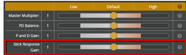
Figure 9: Stick Response Gain slider (FF slider) in PIDs tab
