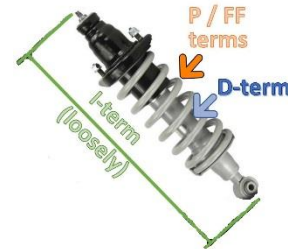
Figure 6: Analog of PID terms
